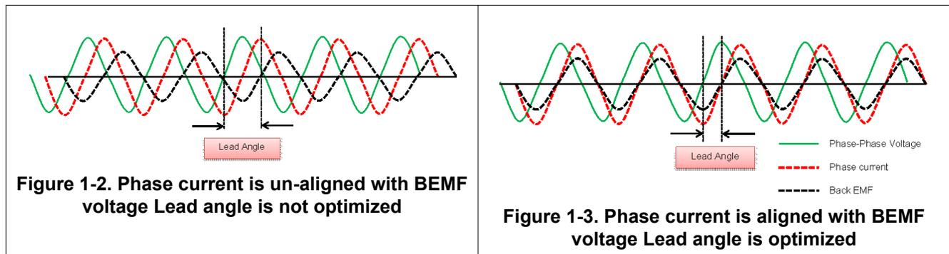
Figure 1-2. Phase current is un-aligned with BEMF voltage Lead angle is not optimized
