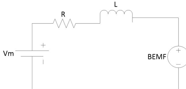
Figure 1-1. BLDC Motor model
