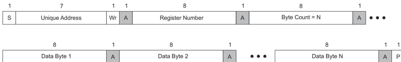
**Figure 1-2. I2C Unique Address Write Register Protocol**
