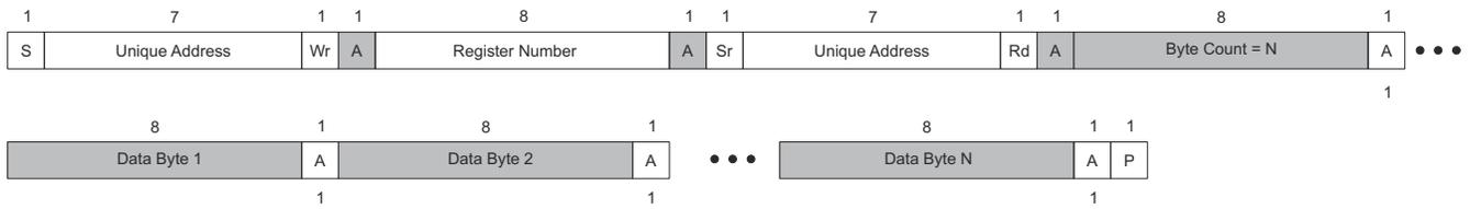
**Figure 1-3. I2C Unique Address Read Register Protocol**
