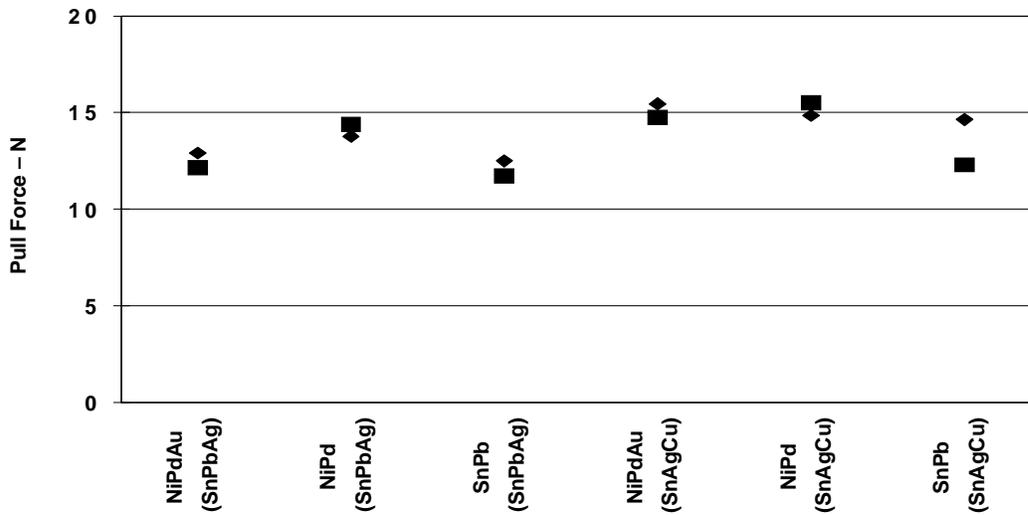
Figure 30. 208 PDV TQFP Lead-Pull Results, NiAu Finish, Before and After Temperature Cycling
