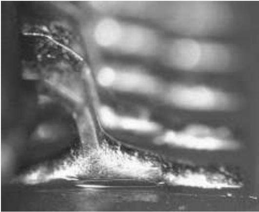
**Figure 21. NiPdAu Finish 208 PDV TQFP, SnPbAg Solder, NiAu PWB Finish**
