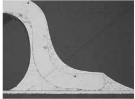
**Figure 32. SnPb SOP, SnPbAg Solder, NiAu PWB Finish, 0 Temperature Cycles**
