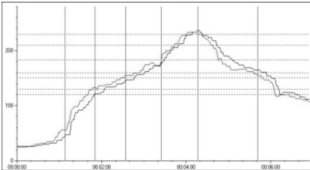
**Figure 8. Reflow Profile for SnAgCu Solder Alloy**
