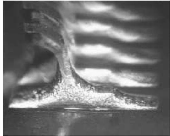
**Figure 22. NiPdAu Finish 208 PDV TQFP, SnAgCu Solder, NiAu PWB Finish**
