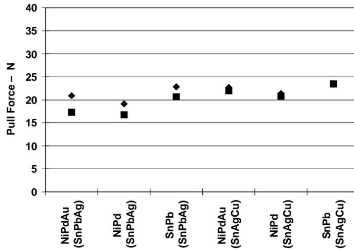
Figure 24. 20 NS SOP Lead-Pull Results, NiAu Pad Finish, Before and After Temperature Cycling
