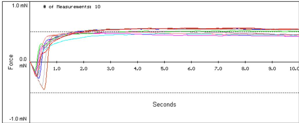
**Figure 4. Wetting Balance Curves for SnPb Component Finish With SnAgCu Solder**
