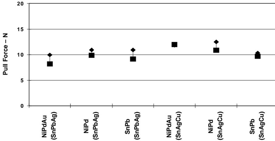
**Figure 25. 176 PBL TQFP Lead-Pull Results, OSP Pad Finish, Before and After Temperature Cycling**
