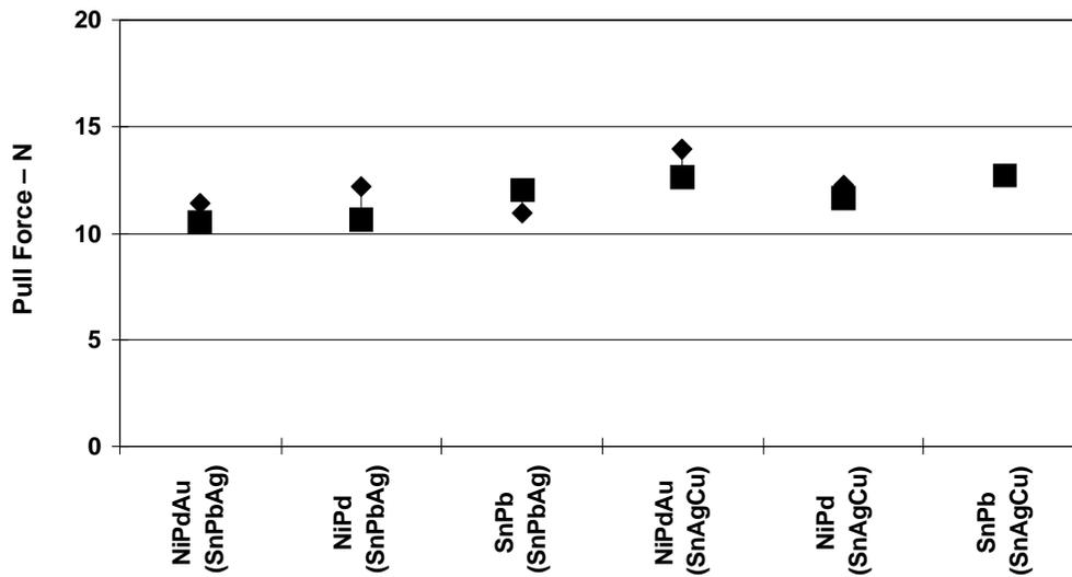
Figure 28. 176 PGF TQFP Lead-Pull Results, NiAu Pad Finish, Before and After Temperature Cycling
