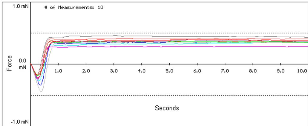
**Figure 5. Wetting Balance Curves for TI NiPd Component Finish With SnAgCu Solder**
