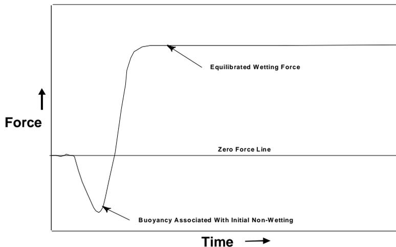
**Figure 3. Typical Wetting Balance Curve**
