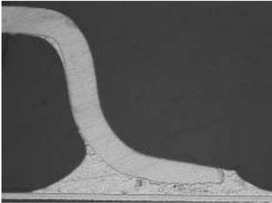
**Figure 31. NiPdAu SOP, SnPbAg Solder, NiAu PWB Finish, 0 Temperature Cycles**
