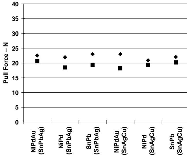
**Figure 23. 20 NS SOP Lead-Pull Results, OSP Pad Finish, Before and After Temperature Cycling**
