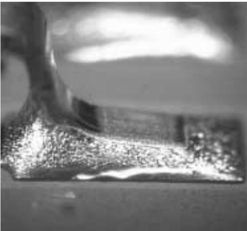
**Figure 13. NiPdAu Finish NS, SnAgCu Solder, NiAu PWB Finish**
