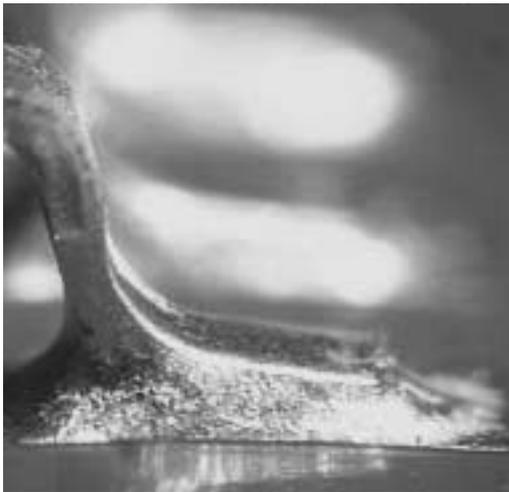
**Figure 9. NiPdAu Finish NS, SnPbAg Solder, NiAu PWB Finish**
