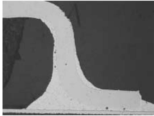
**Figure 38. SnPb SOP, SnAgCu Solder, 1000 Temperature Cycles**
