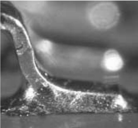
**Figure 11. NiPdAu Finish NS, SnPbAg Solder, OSP PWB Finish**
