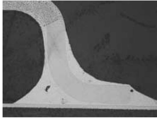
**Figure 36. SnPb SOP, SnAgCu Solder, NiAu PWB Finish, 0 Temperature Cycles**
