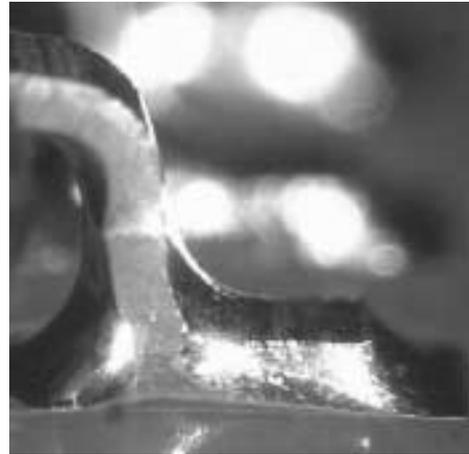
**Figure 12. SnPb Finish NS, SnPbAg Solder, OSP PWB Finish**
