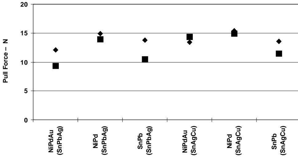
Figure 29. 208 PDV TQFP Lead-Pull Results, OSP Finish, Before and After Temperature Cycling
