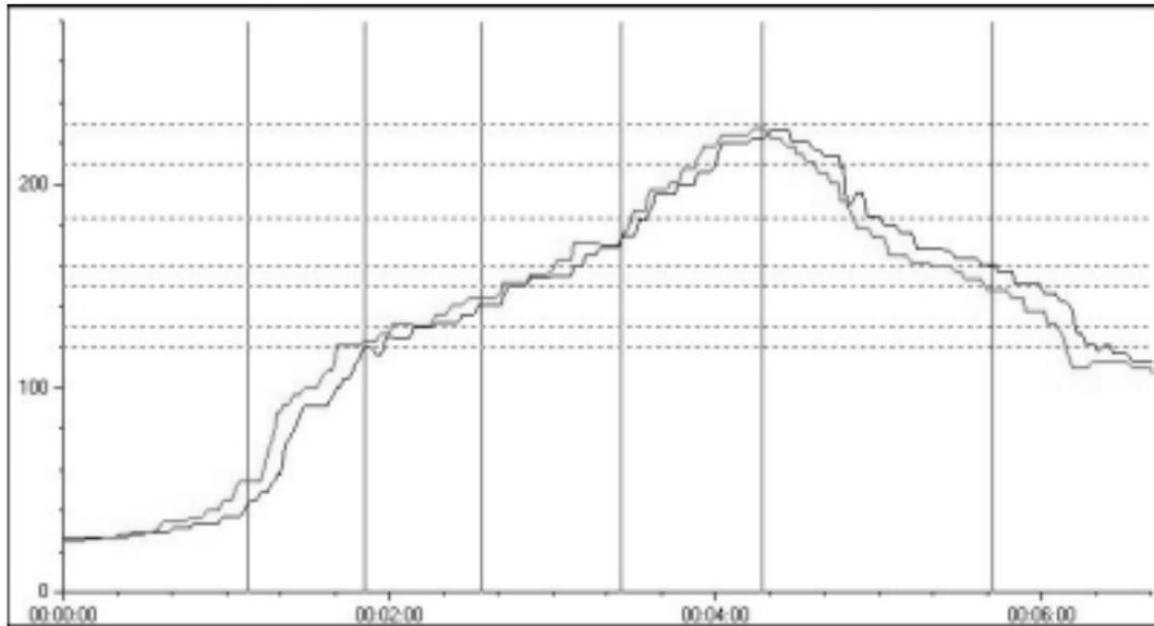
**Figure 7. Reflow Profile for SnPbAg Solder Alloy**
