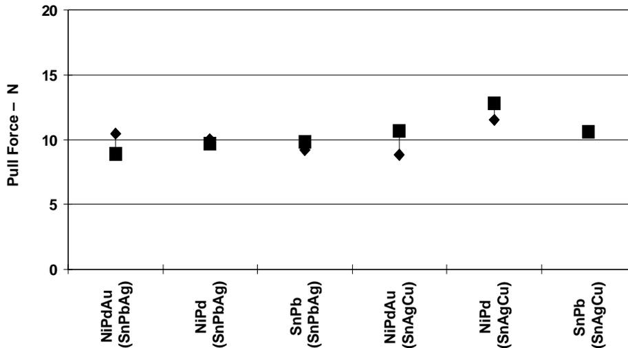
**Figure 26. 176 PBL TQFP Lead-Pull Results, NiAu Pad Finish, Before and After Temperature Cycling**
