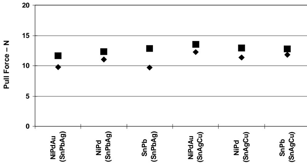
Figure 27. 176 PGF TQFP Lead-Pull Results, OSP Pad Finish, Before and After Temperature Cycling
