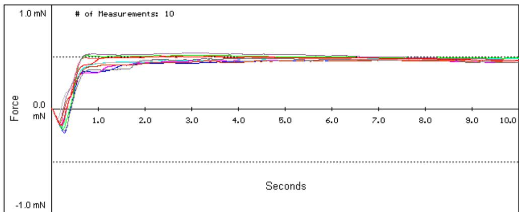
**Figure 6. Wetting Balance Curves for TI NiPdAu Component Finish With SnAgCu Solder**
