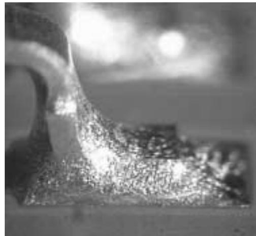
**Figure 14. SnPb Finish NS, SnAgCu Solder, NiAu PWB Finish**
