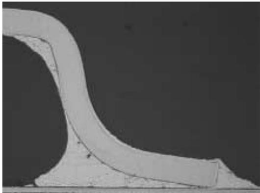
**Figure 33. NiPdAu SOP, SnPbAg Solder, NiAu PWB Finish, 1000 Temperature Cycles**
