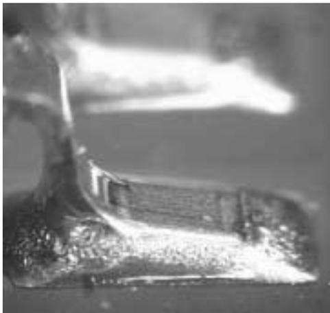
**Figure 15. NiPdAu Finish NS, SnAgCu Solder, OSP PWB Finish**
