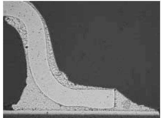
**Figure 34. SnPb SOP, SnPbAg Solder, NiAu PWB Finish, 1000 Temperature Cycles**
