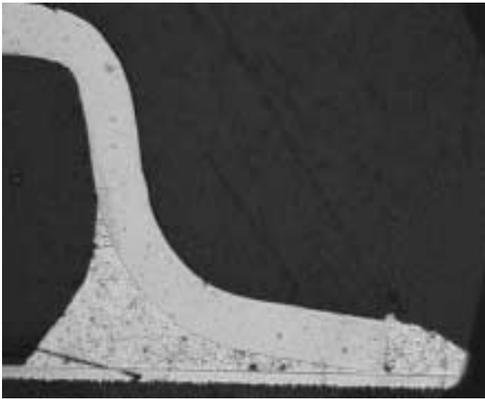
**Figure 37. NiPdAu SOP, SnAgCu Solder, 1000 Temperature Cycles**
