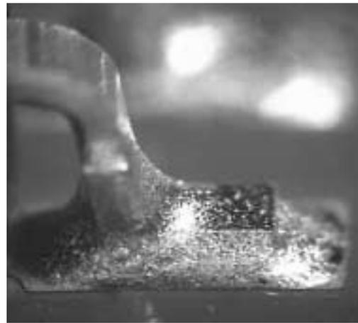
**Figure 16. SnPb Finish NS, SnAgCu Solder, OSP PWB Finish**
