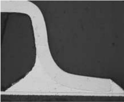
**Figure 35. NiPdAu SOP, SnAgCu Solder, NiAu PWB Finish, 0 Temperature Cycles**
