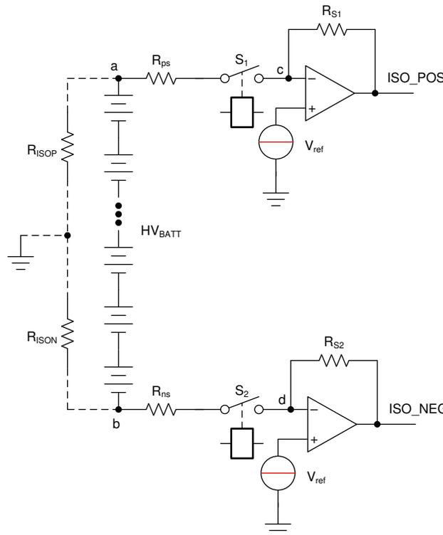
**Figure 2-1. Isolation Errors at Both Positive and Negative Terminals**
