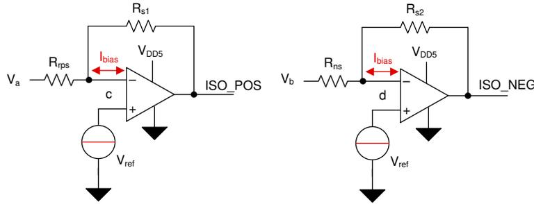
**Figure 4-1. Input Bias Current Flows into or out of Inverting Input**
