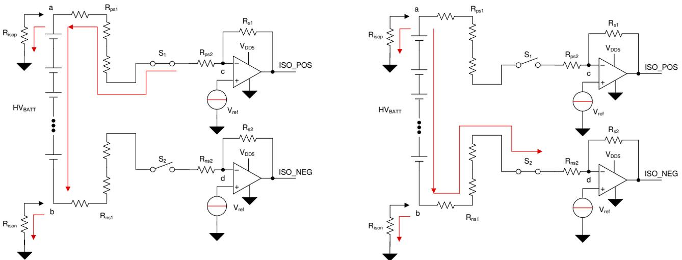
**Figure 2-2. Measurement Procedure: Only One Switch is Closed Periodically**
