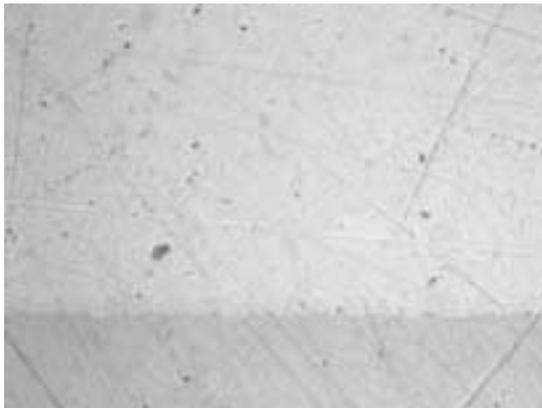
**Figure 24. Sn/Ag/Cu Solder (235°C Peak),
