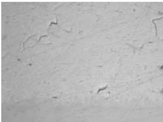
**Figure 26. Sn/Ag/Cu Solder (260°C Peak),
